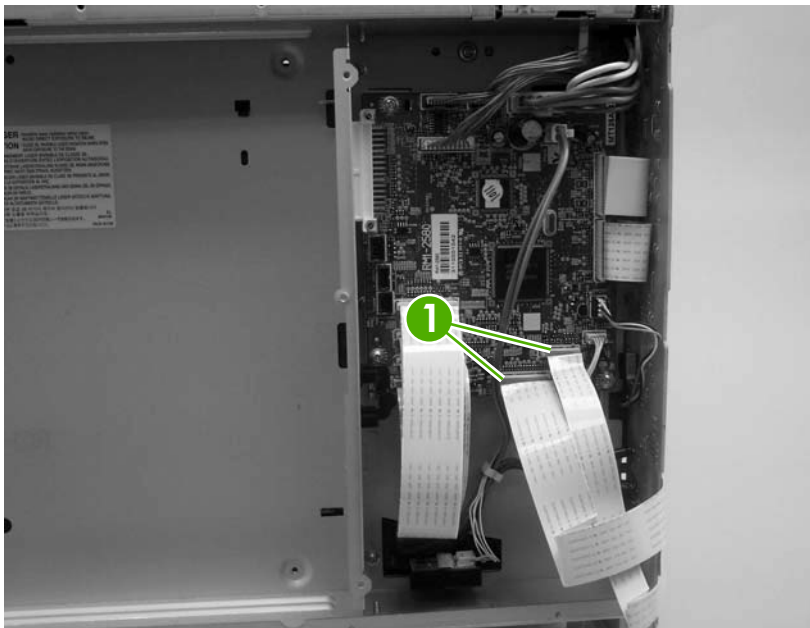
Figure 5-88 Remove the high-voltage power supply (1 of 3)
